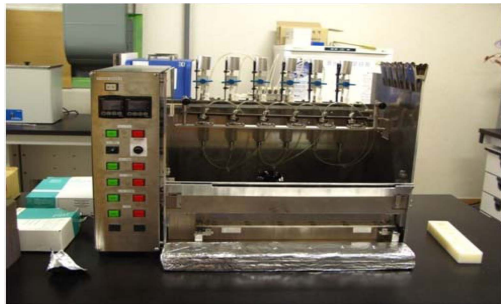
Fig. 3. Rapiana for fast PCBs analysis.
