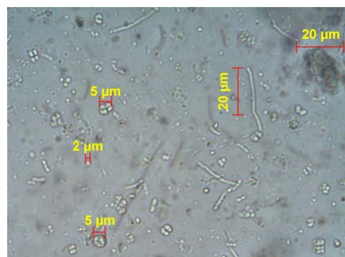
Fig. 2. Microorganisms in the wastewater sludge used in this study (10×40).
