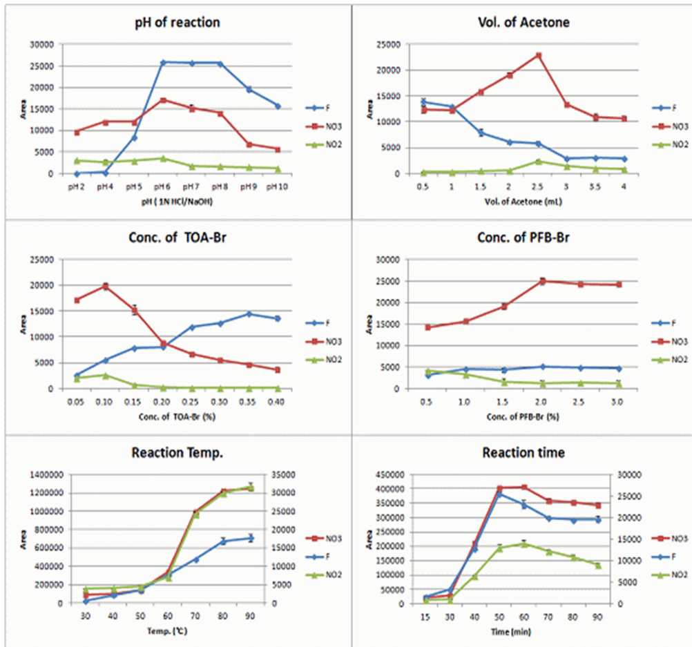
Fig. 2. The condition of reaction of fluoride, nitrite and nitrate with PFB-Br.
