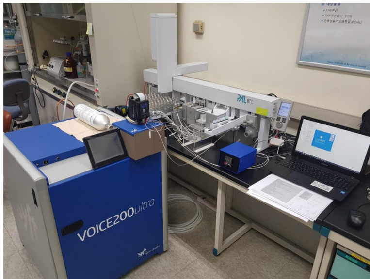
Fig. 1. Configuration of autosampler based online headspace and instrumentation with SIFT-MS.
