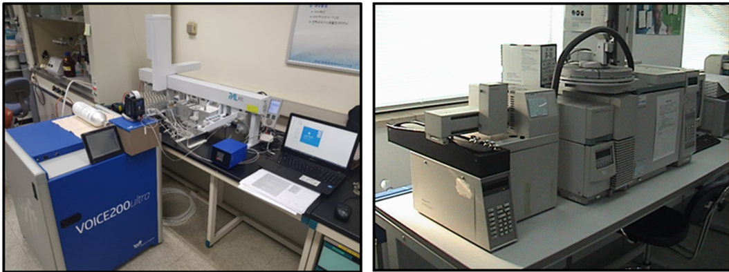
Fig. 1. Online headspace-SIFT/MS system (left) and headspace-GC/MS system.
