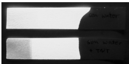
Fig. 2. Detection of TNT in seawater. Two paper tickets were coated with polysilole, then soaked for 30 s in seawater (collected off Scripps Pier, La Jolla, CA). The seawater used in the bottom ticket was spiked with purified TNT. The top ticket is the control. The image was taken under a black light.
