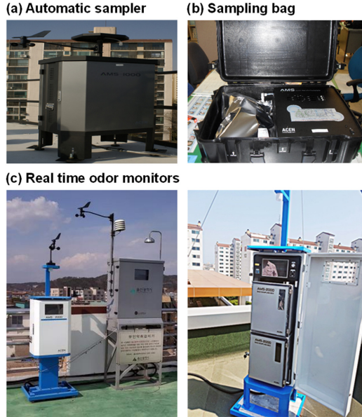
Fig. 3. Sampling devices and real-time odor monitors installed in Ulsan. Photos were obtained from the Ulsan Metropolitan City.
