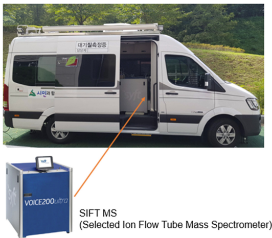
Fig. 5. Mobile monitoring system for the monitoring of odor and VOCs operated by the Ulsan Institute of Health and Environment.
