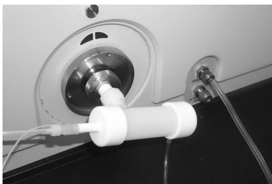
Fig. 1. PFA Spray Chamber and Polyethylene Nebulizer this experiment for HF media sample (This was r KRISS Lab).
